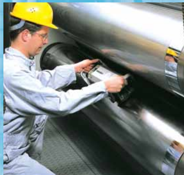
Measuring roller parallelism
