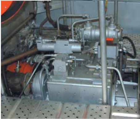
... single-stage spur gear - drive power P = 2320\text{kW} - gear ratio i = 2.58:1
