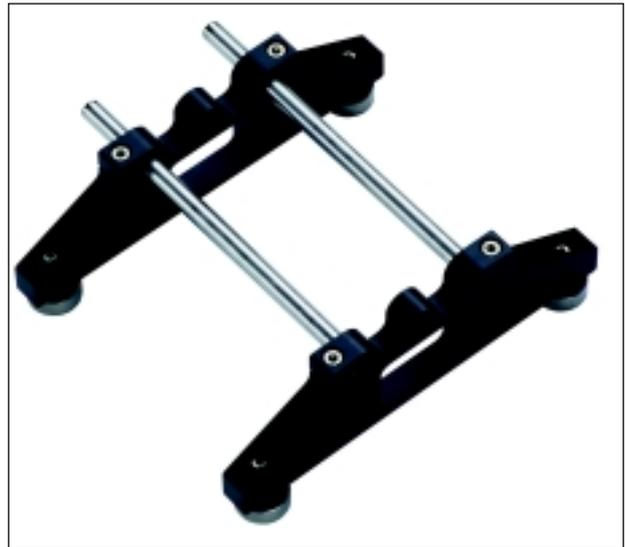
This bracket can replace the compact chain-type bracket for large couplings having correspondingly large bolt holes. Especially handy when radial clearance around the coupling rim is limited, this bracket allows the laser beam to be directed through a coupling bolt hole with the emitter and receiver mounted below the rim.
