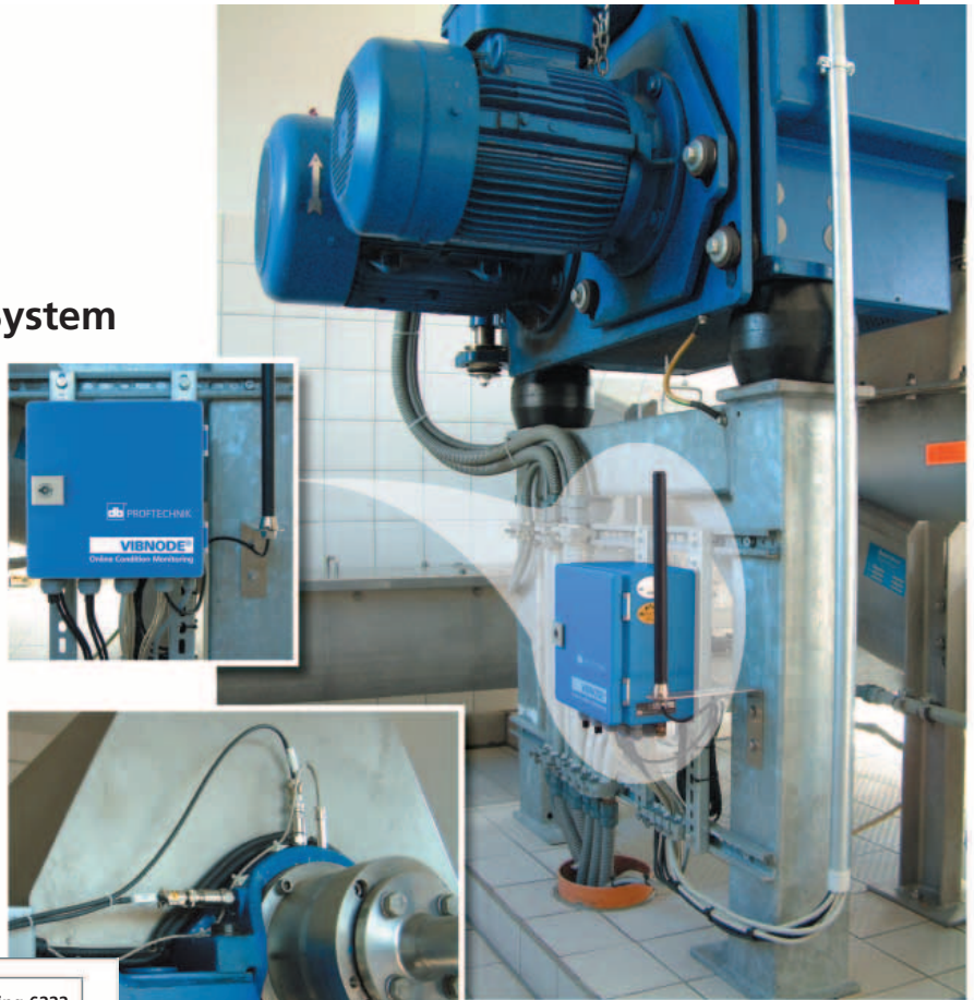
VIBNODE® with integrated GPRS modem and antenna
