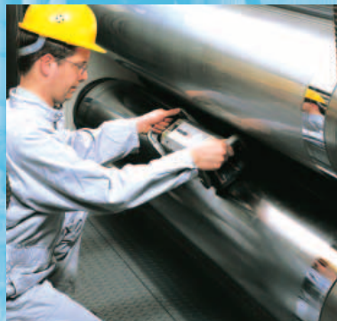
Measuring roller parallelism
