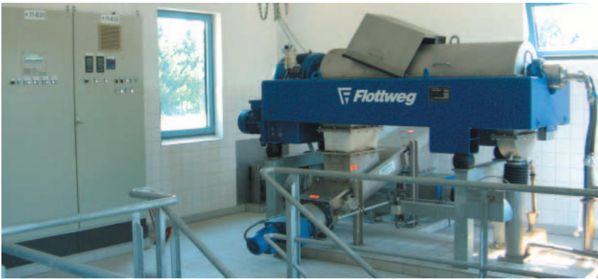
Horizontal solid bowl screw centrifuge for sludge dehydration in a wastewater treatment plant
