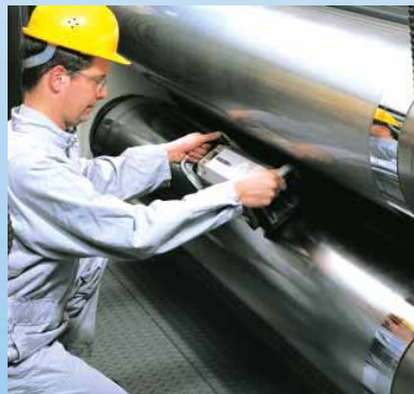
Measuring roller parallelism
