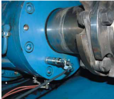
Vibration sensor on drive shaft
