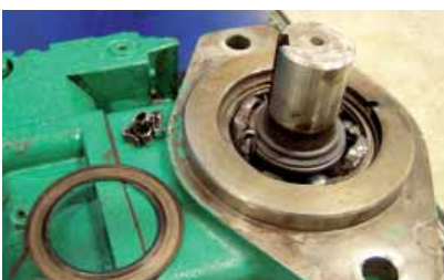
Roller bearing damage (cage damage) on the axial bearing of an axial piston pump
