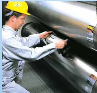
Measuring roller parallelism
