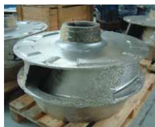
Wear on the pump impeller of an FGD pump due to aggressive media
