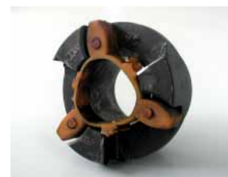
Coupling wear due to faulty shaft alignment
