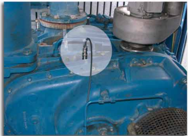
Vibration sensor on bearing of main and secondary rotors
